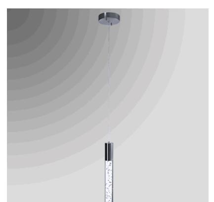
10"H 1-Light Chrome Pendant, direct wired, LED 3 watt, 210 Lumens, CRI 80, 3000K with Bubble Acrylic Diffuser. Cord adjustable to 59" OAH.
